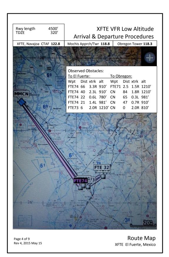
XFTE VFR Low Altitude Rwy length TDZE 4500′ 320′ **Arrival & Departure Procedures** XFTE CTAF 122.8 Mochis Apprch/Twr 118.8 Obregon Tower 118.3 2530 FTE 32 17.7 nm, 229° 210' 15.0 mm. 46° 6.4 nm, 074 1210
