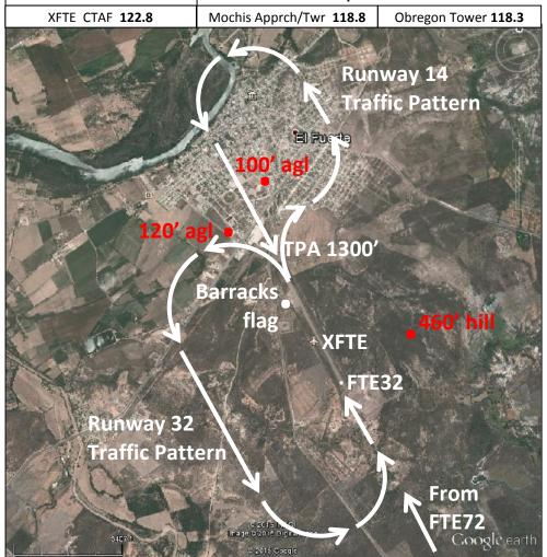
Notes: Highest terrain under course is 460' at 3 nm to FTE72. 460' msl hill right of Rwy 32. Rwy 14 downwind goes to the river for a long, straight-in approach to avoid antennas. The closest antenna at about 120' above the runway may penetrate the rwy 14 arrival slope. Use a Traffic Pattern Alt of 1300'. Use Los Mochis altimeter on arrival.
